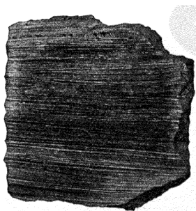
FIG. 116.—Flow-structure in rhyolite, from the north of Ireland (about 1/2).
